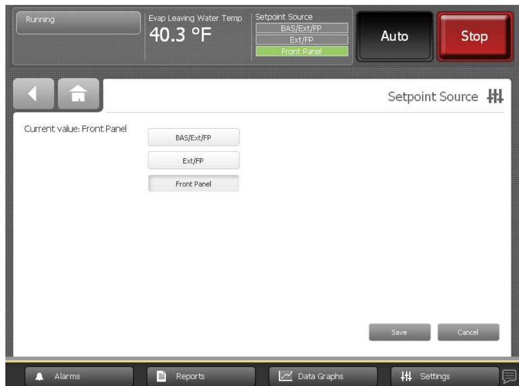
Figure 25. Setpoint Source screen
